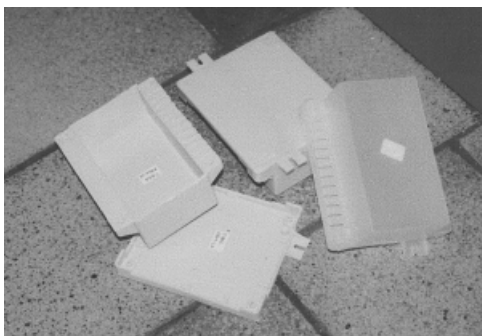
Figure 8 Box and lid produced (less milky: plain PP; more milky: recycled composite).
